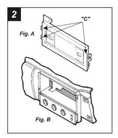
Cut and remove all mounting tabs on the *Radio Housing* EXCEPT tabs "C". (see Fig. A). Using a dremel tool, cut and remove the *shaded* portions of the sub-dash plastic. This will provide the necessary depth for installation. (see Fig. B). Skip to the Installation Instructions for ALL VEHICLES on Page #5.
